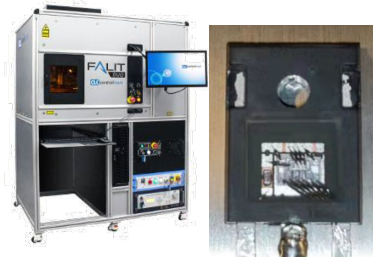
Figure 11. Laser machine (left). Decapsulated device using laser (right).
