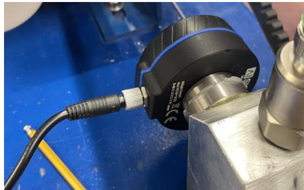
Figure 12: Vibration sensor (Case 2 demonstration setup Küffer Elektro-Technik AG)
