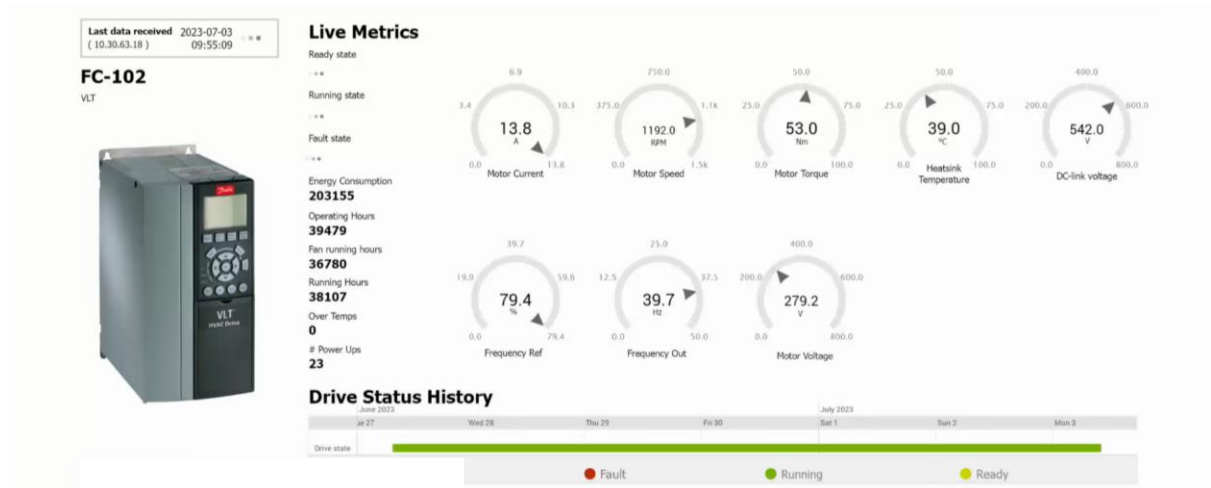
Figure 7 Example for data delivered by a VSD (source: Danfoss)
