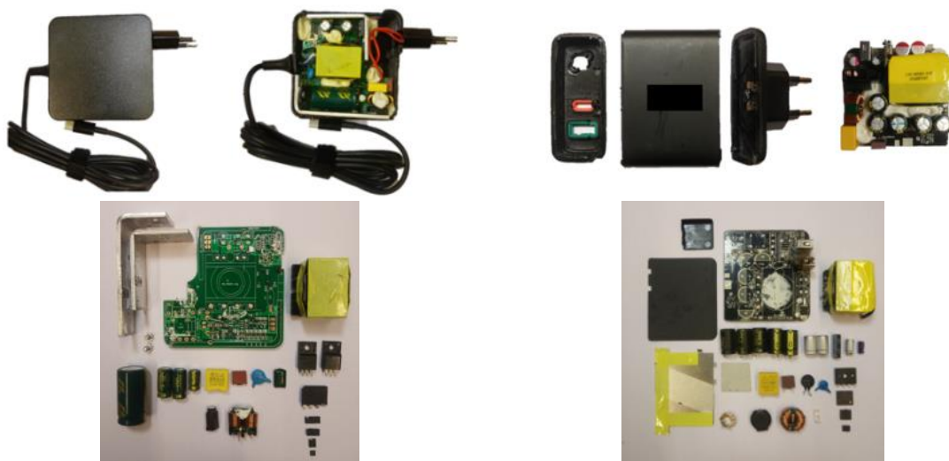
Figure 4: Laptop chargers investigated, on the left a 60W Si-based charger (reference), and on the right a 60W GaN-based charger [16]
