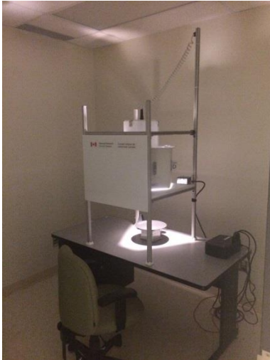
Figure A1. Images of the NRC apparatus installed in the test room. For the image on the left, the hallway outside provided ambient light for the photograph, but the door was closed during testing. The image on the right shows the desk surface as seen by the participant.
