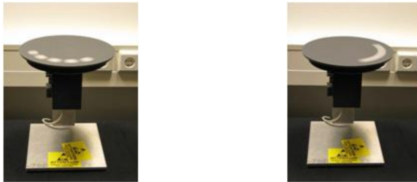
Figure A4. These images from Reference 17 demonstrate the stroboscopic effect. When one sees this effect, the moving disk looks like the image on the left. With no stroboscopic effect, it looks like the disk on the right.
