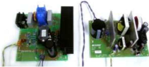
ON Semiconductor PFC (left) and Power Integrations SMPS (right).
