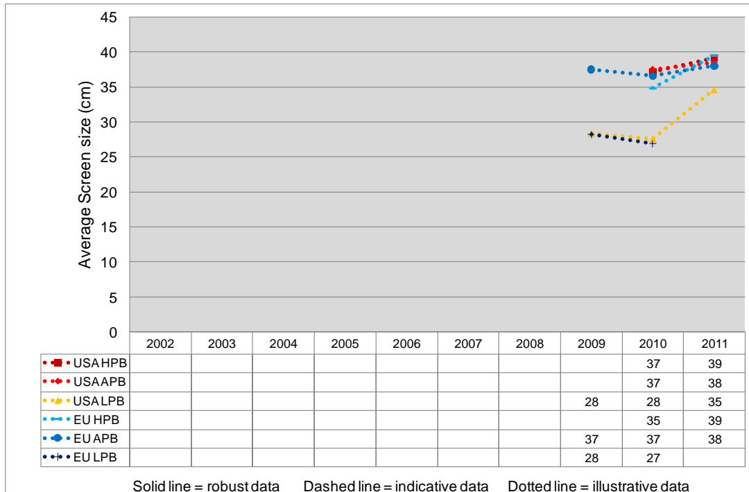
Figure 31. Average screen size (cm) for the 3 performance bands for USA and EU ENERGY STAR.
