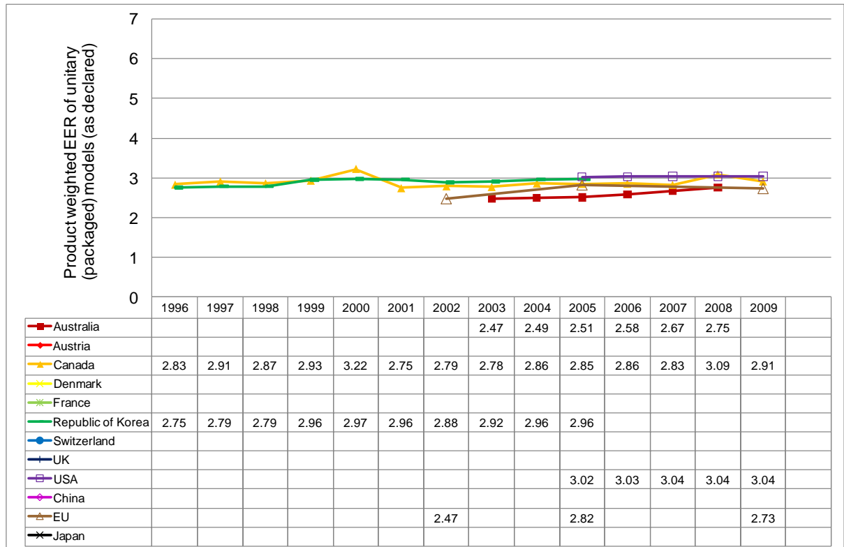
Figure 23. Product weighted energy efficiency ratio (EER) for unitary products including USA data.
