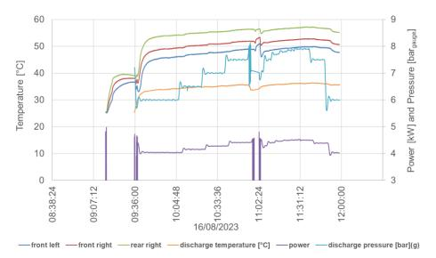
Testing of compressor to be performed not only at a single pressure, but over a number of pressure points including the maximum pressure and in during idling. However without overwriting data in the control system, tests at maximum pressure is impossible, as compressor automatically unloads, if maximum pressure is reached.
