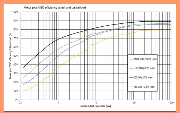
Efficiency for electric motor plus VSD from 0.1 to 1000 kW in full and partial load (source of data: IEC 60034-31 and IEC 61800-9-2)
