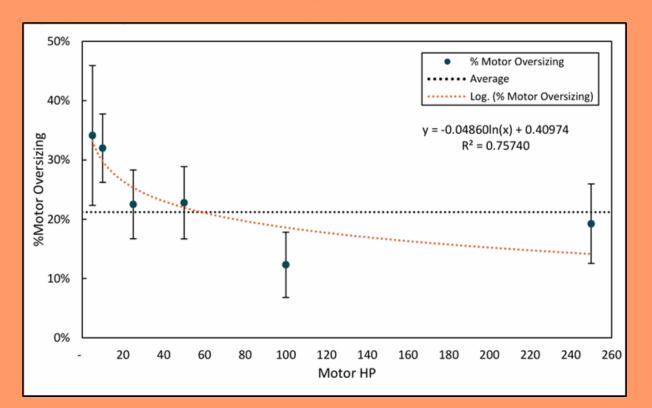
Motor oversizing (%) vs. motor output power (kW), based on analysis of 342 clean water pumps (source of figure: [13] NEEA 2019)
