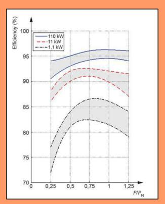
Typical efficiency versus load curve bands, performance characteristics of 4-pole, three phase, cage induction motors of different power ratings, (source: IEC TS 60034-31, edition 2, 2021)
