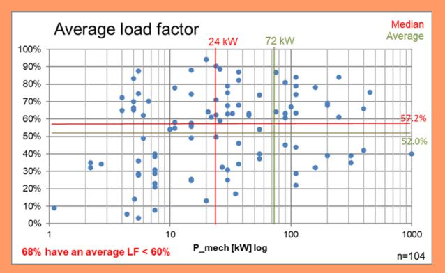
Average load factor (x-axis: 0-100%) of 104 measured motor systems
