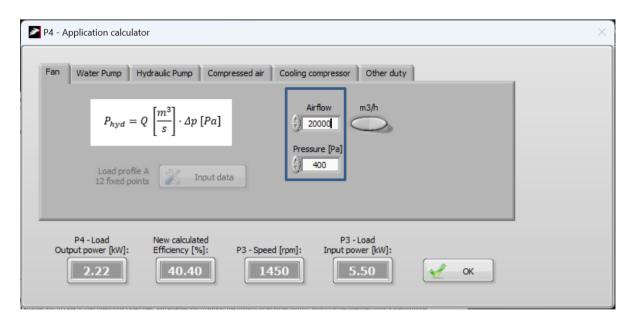
The MST will use this information to calculate the motor loading based on the duty point of the load.
