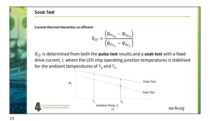
Pulse Test is a proxy for LED chip junction temperature
