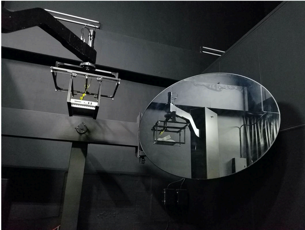
Figure 4-1. A photo of the goniophotometer at KILT
