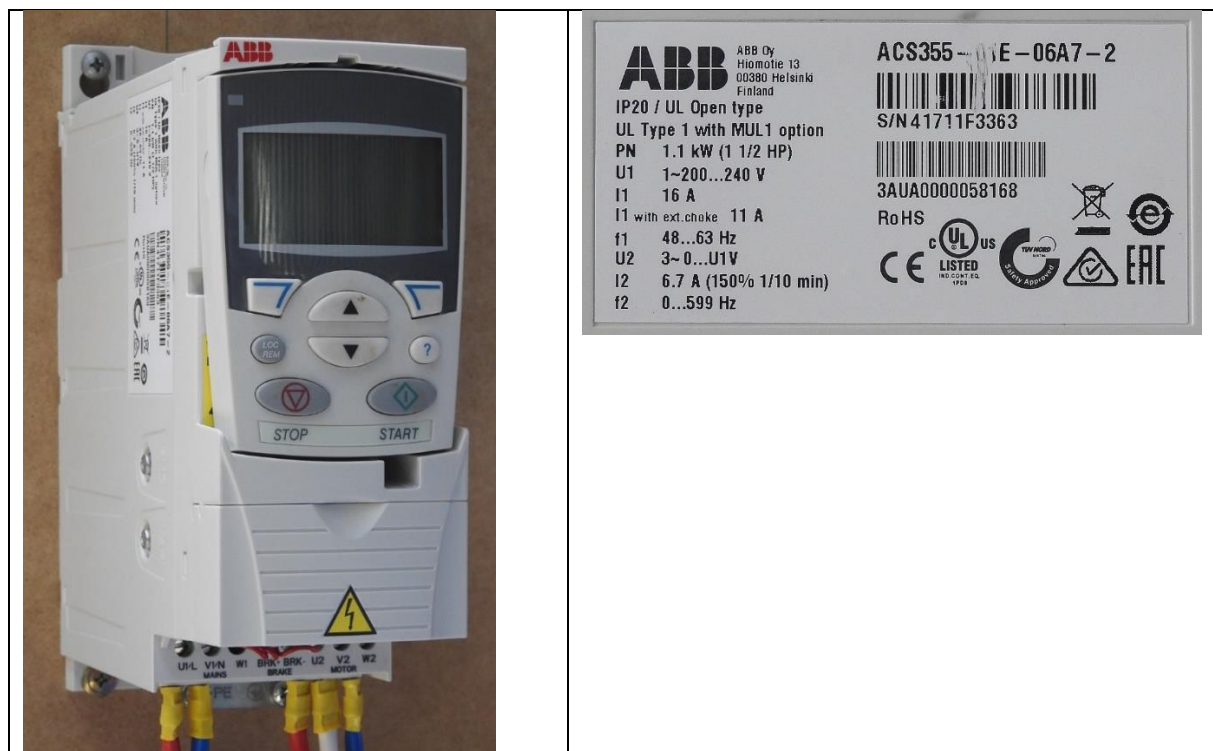
Figure 42 No. 1A: external view and rating plate
